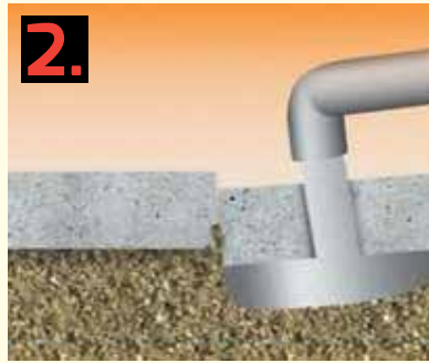
2. Stabilizing grout mixture is pumped under the slab raising it.
