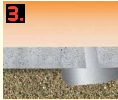
3. The holes are patched with a concrete mix.
